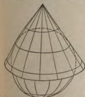
Showing how a map is made by conical projection.
